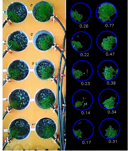
Fig. 5. Half of the RAPID-MOLT pots shown on the 8th day of the experiment monitoring grass growth under variable irrigation. The figure shows the raw RGB image (left side) from which the leaf masks and LAI values for each pot (right side) are extracted. The bottom left pot received 0.72mL of irrigation, increasing up to 1.41mL for the top left, continuing with the second column upwards ending at 2.08mL at the middle top right pot. The right part shows the left RGB image processed via the data pipeline. As can be seen the LAI values correlate positively with the daily applied irrigation input.
