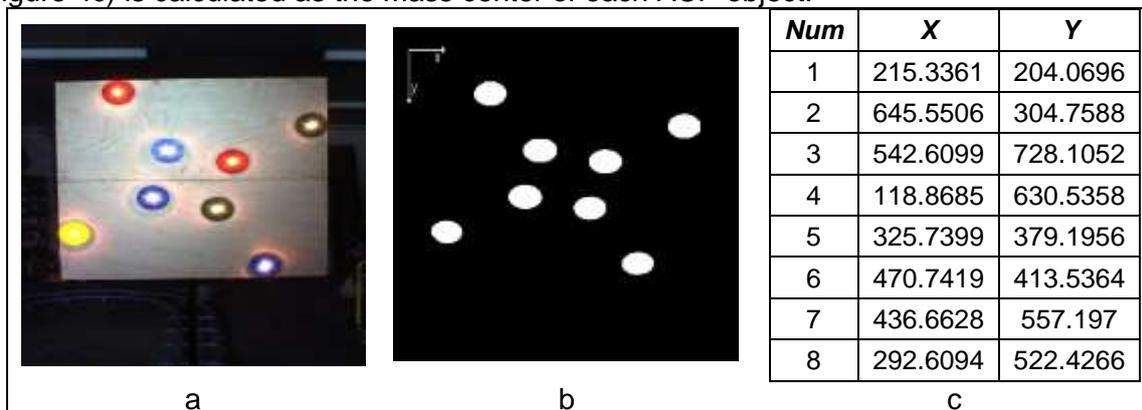
Figure 4 – (a) Visual image, (b) RGB ACP's positions, (c) ACP's position (sort according to Figure 2a)
