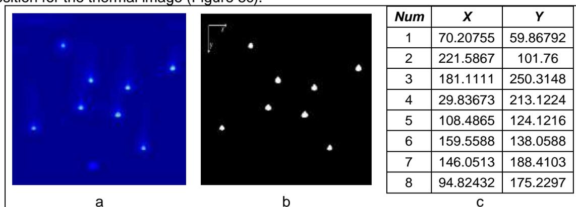
Figure 5 - (a) Thermal image, (b) Thermal ACP's position, (c) ACP's position (numbers according to Figure 2a)
