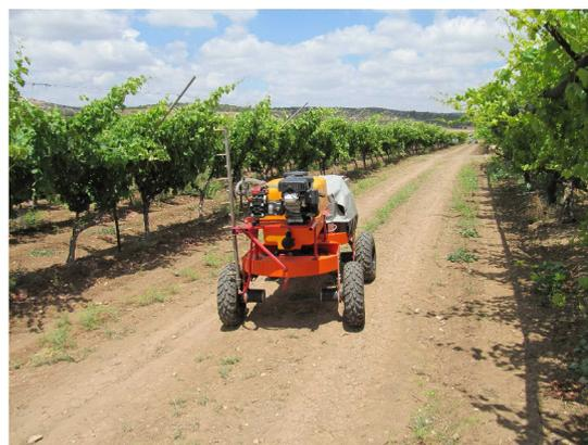
Fig. 5 - Robotic sprayer (Berenstein et al., 2010)
