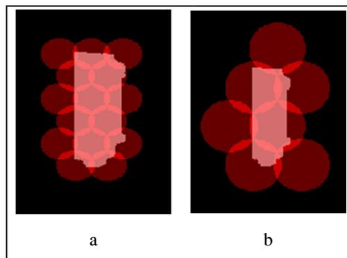
Fig. 4 - Spray diameter, (a) small diameter, (b) large diameter
