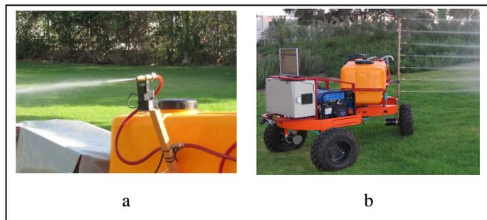
Fig. 6 – (a) Pan\Tilt head with spraying nozzle attached, (b) spraying boom with spread nozzles
