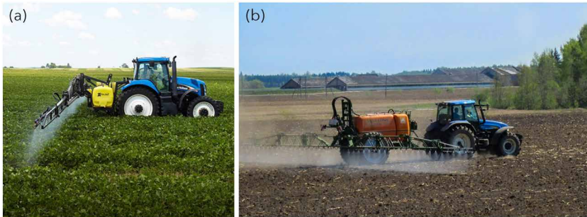
Figure 1 Tractor sprayers. (a) The sprayer is mounted directly on the tractor (also known as three-point sprayer), (b) trailed sprayer where the sprayer is being towed by the tractor.
