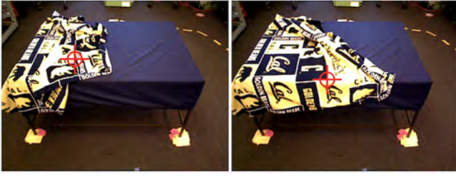
Fig. 14: Left: the RGB-based grasping policy selects a grasp point at a spot in the lower left and somewhat far from the actual blanket corner. Right: after grasping and pulling, the RGB-based policy continues to pick points near the lower-center portion of the blanket, which results in no additional coverage for that side. The grasping point determined from the RGB-based policy is shown with the red cross hair. See Figure 15 for a third-person view of the robot when it executes the grasp at the image to the right.
