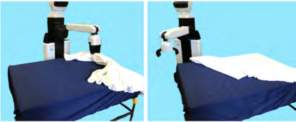
Fig. 7: The analytic baseline can often do reasonably well because the white blanket is smooth and stretchy. While the initial pull above achieves reasonable coverage, it covers a blanket corner and makes it harder for subsequent grasps and pulls to make nontrivial coverage progress.
